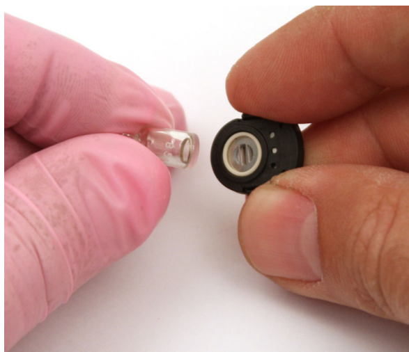
Figure 28: Reinstalling the Electrode Lamp
