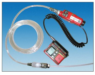
The GX-2001 is the smallest 4-gas monitor in the world and now it is available with a compact battery operated sample-drawing pump that attaches in line for remote, portable monitoring. Together the model RP-6 sample drawing pump and the GX-2001 make a complete solution for confined space entry situations.
