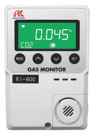
RKI is pleased to introduce the RI-600 stand-alone Carbon Dioxide monitor. The RI-600 uses NDIR technology to detect Carbon Dioxide in five different ranges including PPM and % volume. Its sleek, lowprofile design is equipped with a unique tri-color display which changes color as Carbon Dioxide levels reach each alarm level.
